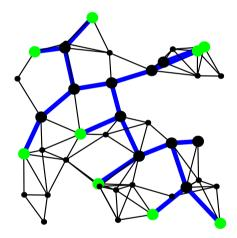
Figure 3.3: A multicast tree minimizing the number of retransmissions in a wireless multihop network.
