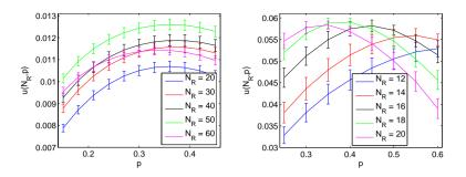
Figure 3.4: The maximum packet flow for deterministic forwarding (left) and opportunistic forwarding (right).
