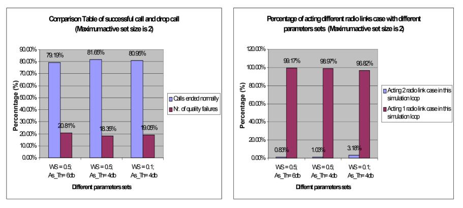
Simulation result of different parameter sets of "Window-average algorithm" (AS=2)
