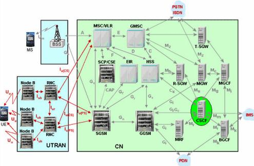
Main network elements of the UMTS release 5 architecture
