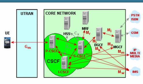
Main IMS network elements that use SIP signalling
